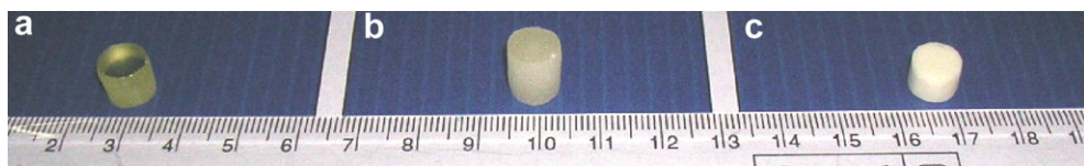
Fig. 3. Hand specimens of thoria glass samples loaded with 15.87 wt%, 18.61 wt% and 23.75 wt% thoria respectively showing (a) transparent, (b) translucent and (c) opaque optical properties.
